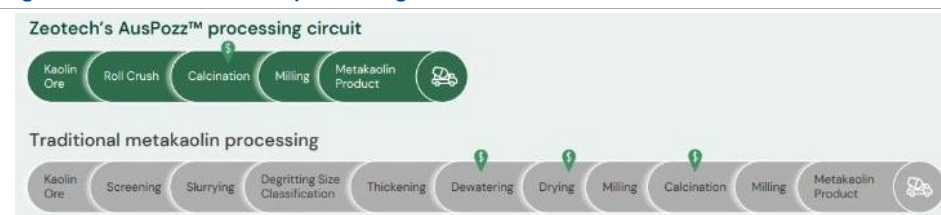
Figure 13: ZEO's AusPozz™ processing circuit
